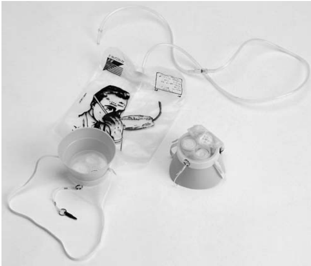
FIGURE 2-15 Passenger oxygen mask. (Courtesy of B/E Aerospace.)
